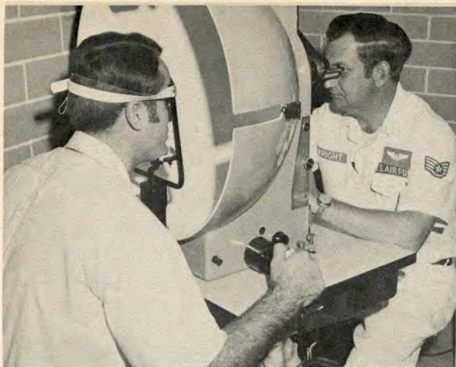
A special piece of equipment at USAFSAM is the Goldmann perimeter for the detection of any impairment in a pilot's field of vision. This study is being conducted by SSgt Dean Wright of the Ophthalmology Branch.
